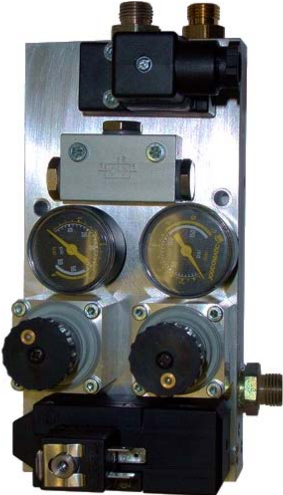
Fig.07 - Low Pressure System (ref. 4.17.00.01)
